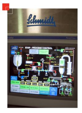
candy wrapper. Therefore, it is necessary to remove the water through evaporation so it can become more viscous and easily wrapped. The higher temperatures help keep the sugar solution flowing while the water is removed. Once the solution is at the proper concentration, or low level of water, it is cooled and formed into round candy shapes before it is wrapped.
