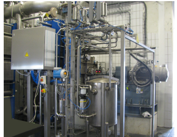
SIGMASTAR 90V MVR – Evaporating capacity: 2.000 kg/h
