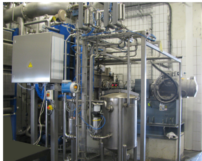
SIGMASTAR® 90V MVR – Evaporating capacity: 2.000 kg/h
