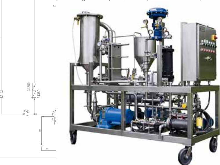
1-stage SIGMAVAP Pilot Plant various products - evaporating capacity up to 50 kg/h
