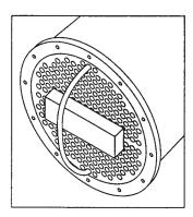
The bundle should be supported on the tube baffles, supports, or tubesheets to prevent damage to the tubes. The gasket and packing contact surfaces should be protected.
