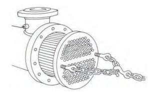
Cables may be threaded through several tubes (tube diameter permitting) and pulled. The cable must be passed over a wooden block at the tube ends to protect such tube ends from damage.
