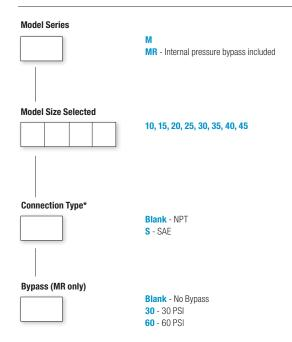
This is a partial flow pressure bypass only. It is not designed to be a full flow system bypass.
