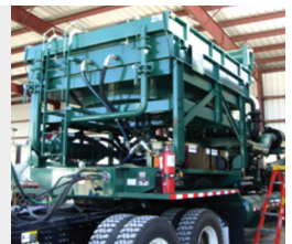
Custom horizontal well frac cooling module for Cummins QSK50
