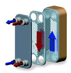
Brazed plate heat exchangers feature corregated stainless steel plates that produce highly turbulent counter-current flow. The result is high heat transfer rates and unmatched efficiency.
