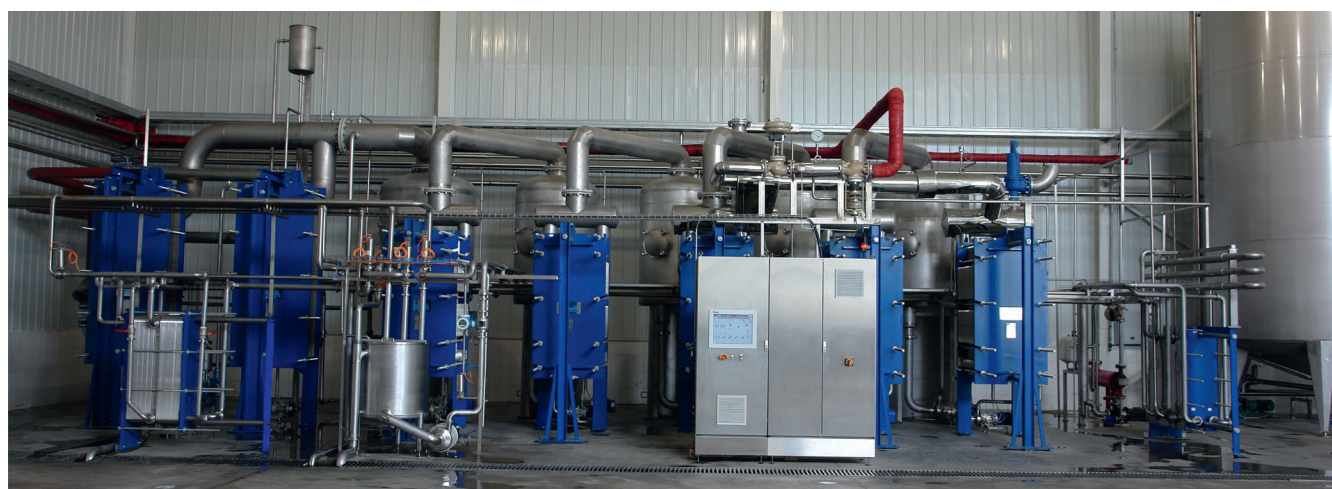
5-stage SIGMASTAR® 90V Evaporating Plant with thermal vapor compressor for apple juice - evaporating capacity 20,000 kg/h
