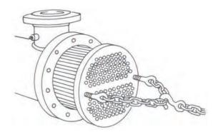
Cables may be threaded through several tubes (tube diameter permitting) and pulled. The cable must be passed over a wooden block at the tube ends to protect such tube ends from damage.
