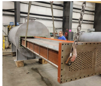
Dual-Circuit ES Cooler Bundle Insertion
